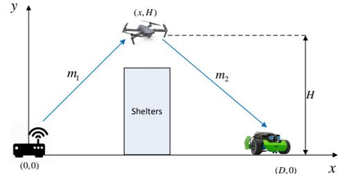
Fig. 1: UAV relay system for delivering URLLC services.
