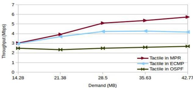
Fig. 8. Throughput of Tactile traffic for different routing protocols
