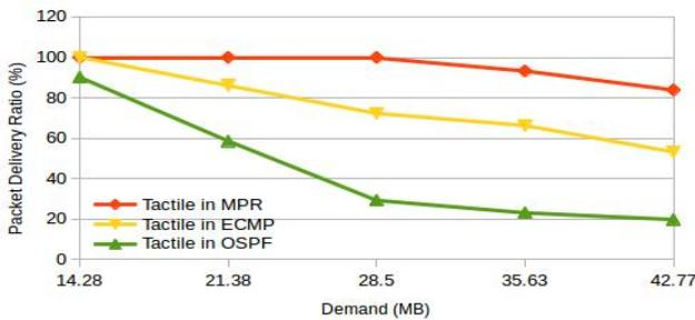
Fig. 7. PDR of Tactile traffic for different routing protocols
