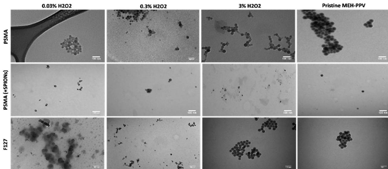
Fig. 4 TEM images of the oxidised MEH-PPV, Taken at 100 $\times$  resolution (scale bar = 100 nm). Top line is oxidised MEH-PPV:PSMA NPs, middle line is oxidised MEH-PPV:PSMA:SPIONS, and bottom line is oxidised MEH-PPV:F127.
