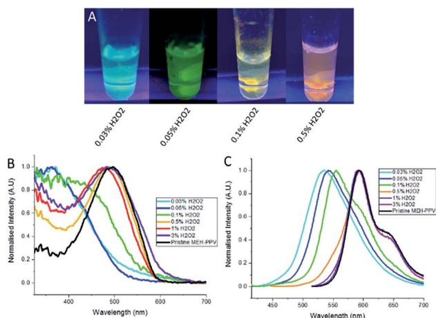
**Fig. 3** (A) Photograph shows emission colours of the different oxidised MEH-PPV:PSMA NPs with SPIONs at  $10 \mu\text{g mL}^{-1}$  against a magnet (excitation at 365 nm). (B) Normalised absorption spectra of oxidised MEH-PPV nanoparticles (+SPIONs), and (C) normalised photoluminescence spectra of oxidised MEH-PPV nanoparticles (+SPIONs). Excitation was either at 365 or 500 nm.
