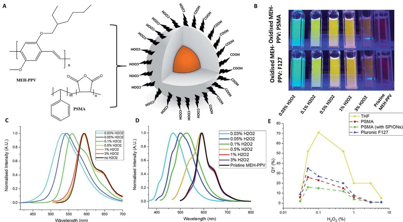
**Fig. 2** (A) Schematic of oxidised MEH-PPV:PSMA nanoparticles. (B) Images of oxidised MEH-PPV incorporated in PSMA nanoparticles or Pluronic F127 micelles. Normalised photoluminescence spectra of oxidised MEH-PPV:PSMA nanoparticles (C) and MEH-PPV:Pluronic F127 nanoparticles (D) (excitation either at 365 or 500 nm). (E) QY% of oxidised MEH-PPV nanoparticles compared to THF solutions.
