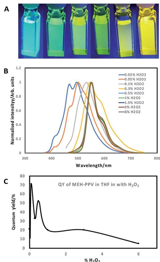
Fig. 1 (A) Images of oxidised MEH-PPV stock solution in THF; (B) normalised emission spectra of oxidised MEH-PPV in THF following 7 days incubation with  $\text{H}_2\text{O}_2$  at different concentrations (excitation 365 nm); (C) QY% of oxidised MEH-PPV in THF.
