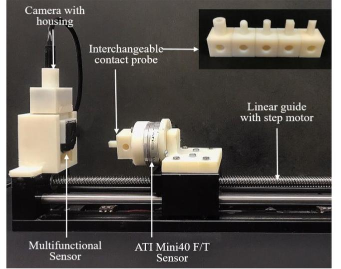
Fig. 3 Contact shape and force experimental setup
