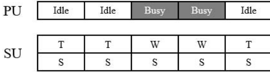
Fig. 4. Listen-And-Talk protocol, where ‘S’, ‘T’ and ‘W’ refer to the sensing period, transmission period and waiting period, respectively.
