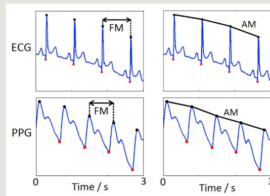
PPG and ECG signals were band-pass filtered (6 – 60 rpm). AM and FM signals were extracted as shown. BW was extracted by decimating the signals to 5 Hz using a low-pass filter below 50 rpm. Only high quality 30 s windows were used.
