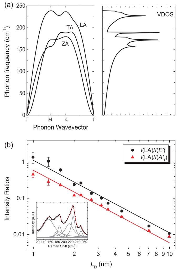
FIG. 3. (Color online) (a) Phonon dispersion and vibrational density of states of 1L-MoS<sub>2</sub>. (b) Experimental intensity ratios  $I(\text{LA})/I(A'_1)$  and  $I(\text{LA})/I(E')$  are reported in symbols. The error bars represent the standard error from the fitting process. The solid lines are linear fits with slope equal to  $-2$ . The low frequency bands, where the LA peak is located at  $\sim 227 \text{ cm}^{-1}$ , are shown in the inset, along with the corresponding Lorentzian fits.
