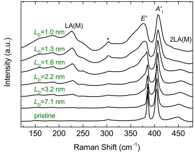
FIG. 1. (Color online) Raman spectra of 1L-MoS<sub>2</sub> flakes with varying interdefect distances  $L_D$ . The asterisk refers to the 2TA(X) Raman peak of the Si substrate. The spectra have been normalized to the intensity of the  $A'_1$  peak, as seen from the relative increase of 2TA(X) with decreasing  $L_D$ .
