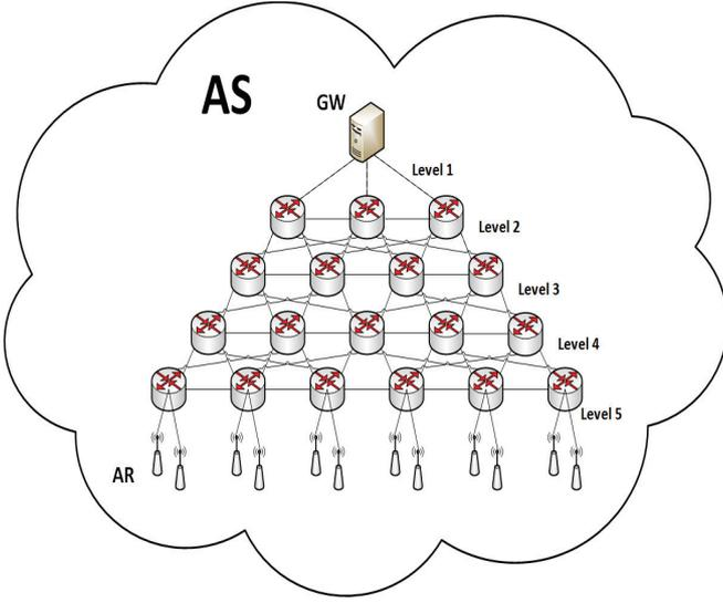
Fig. 1: Autonomous system comprised of 32 nodes and 67 links. Average node degree: 4.19. Total capacity (Gb): 18.40
