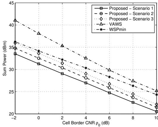
Fig. 4: Sum power versus border CNR,  $\rho_0$ .
