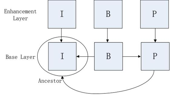
Figure 2. GoP structure with frame dependencies [3].
