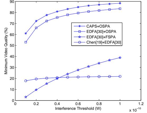
Figure 5. Minimum video quality vs. interference threshold.
