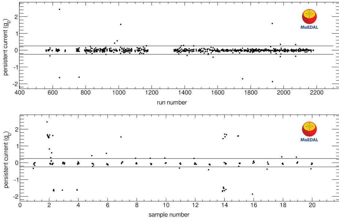
FIG. 1. Top: persistent current (in units of  $g_D$  after application of a calibration constant) after first passage through the magnetometer for all samples. Bottom: results of repeated measurements of candidate samples with absolute measured values in excess of  $0.25g_D$ .
