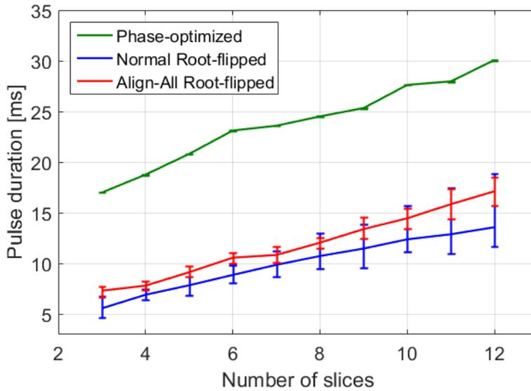
Figure 5 – Duration comparison between phase-optimized, normal root-flipped and align-all root-flipped pulses. For refocusing pulses, the average duration increase is 19.6%.
