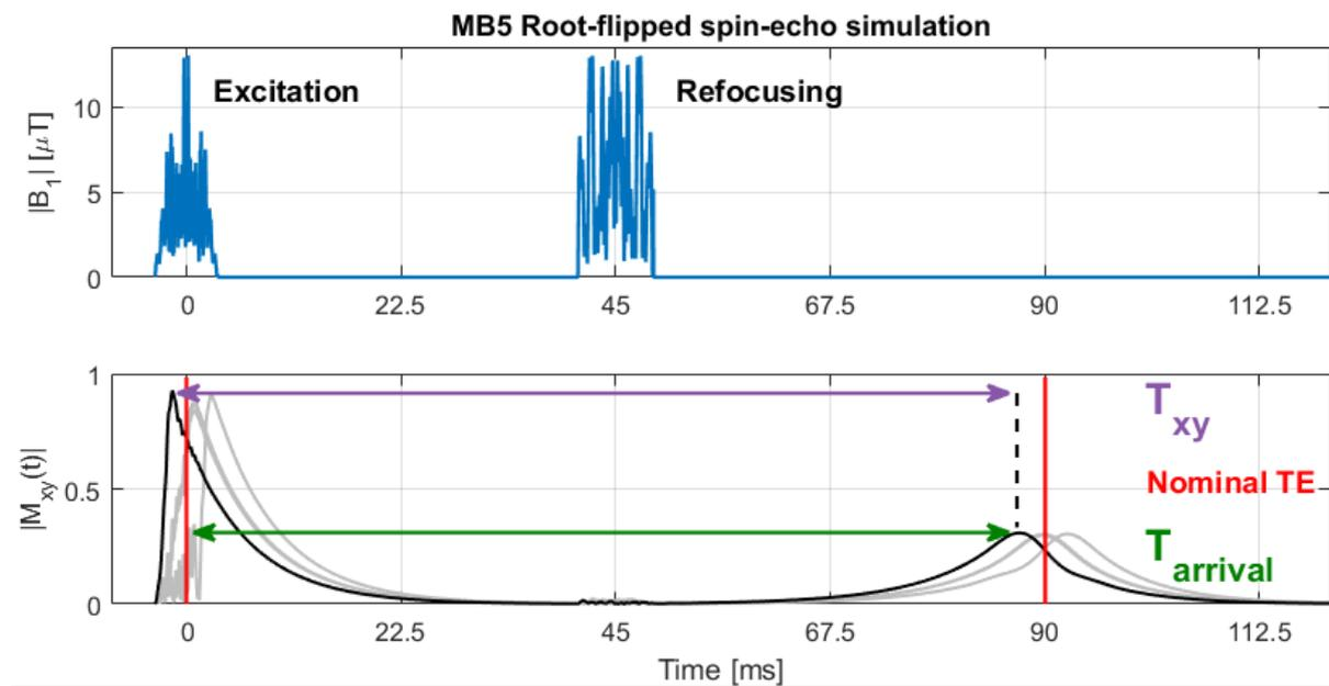
Figure 1 – Top: RF excitation and refocusing pulses (root-flipped design with 5 slices) for a nominal TE of 90ms. Bottom: Transverse magnetization as a function of time for the five slices.  $T_{xy}$  is the time from excitation to the moment the slice fully refocuses.  $T_{arr}$  is the time from the center of the excitation pulse to the moment the slice fully refocuses. For conventional spin-echo sequences these two values are equal to the nominal echo-time.
