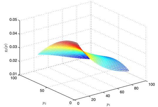
(b) Relation between gravity parameter  $\mathbf{g}_2(p)$  and joint state  $p$
