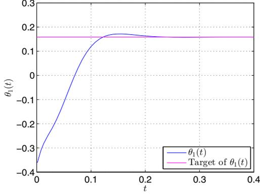
(a) Dynamic trajectory of joint angle  $\theta_1(t)$  under the given control parameter  $k_1$  and  $k_2$
