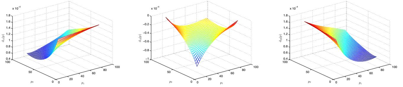
(a) Relation between the inertia parameter  $d_{11}(p)$  and joint state  $p$  (b) Relation between the inertia parameter  $d_{12}(p)$  and joint state  $p$  (c) Relation between the inertia parameter  $d_{22}(p)$  and joint state  $p$
