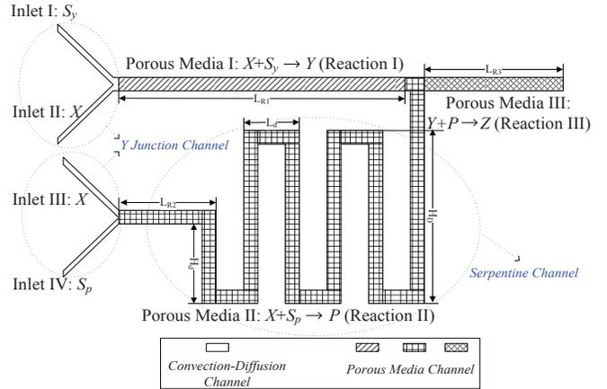
Fig. 3. Novel Microfluidic Device for Pulse Generation.
