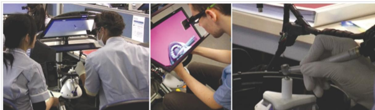
**Figure 1.** Virtual hapTEL simulator (top), with (bottom, left to right) student pair working at the device; view into the virtual mouth; and dental handpiece connected to the device
