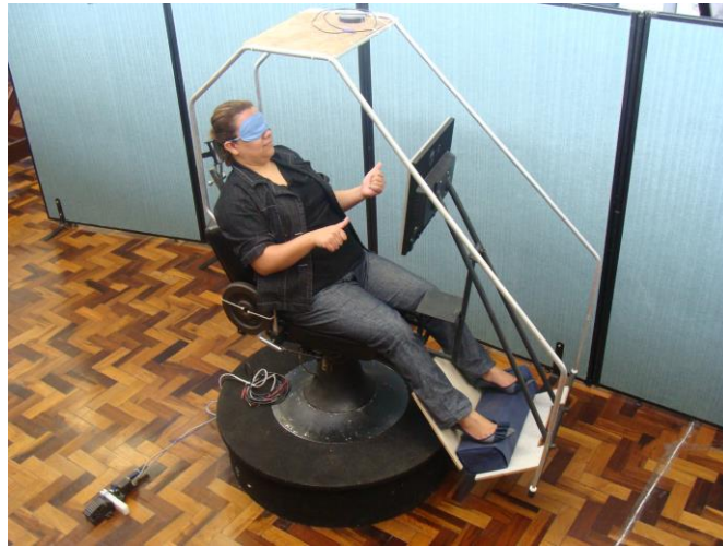
Figure 1. Volunteer in a Barany's Chair at the Microgravity Centre, PUCRS, Brazil . Note that the volunteer is blindfolded to avoid visual inputs during neurovestibular angular acceleration (Source: authors).
