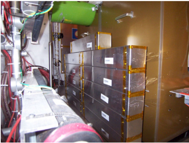
Fig. 5 A photograph of the prototype MMT detector deployed at IP8
