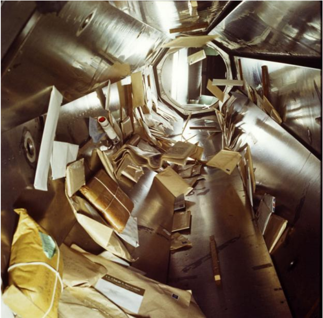
Figure 1.6: Interior of Segregator Drum (SEG) 90
