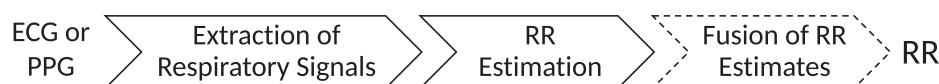
Figure 2. The three stages of a respiratory rate (RR) algorithm, which estimates RR from either the ECG or the PPG. The dashed stage is optional. Adapted from Pimentel et al (2015).
