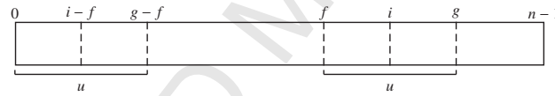
(a) String x = x[0..n - 1] , u occurs at positions 0 and f , and \text{WP}[f] = |u|
